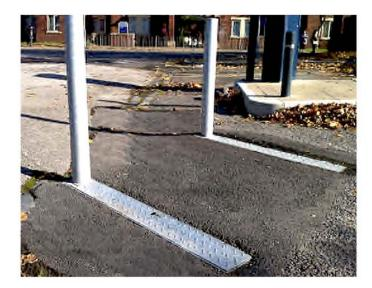
This bollard is a simple solution for parking bay protection and similar applications. The bollard is housed in a recessed casing to eliminate any tripping hazard when the bollard is retracted. The hinged lid is fitted with a cam lock to secure the bollard in either the raised or recessed position.
